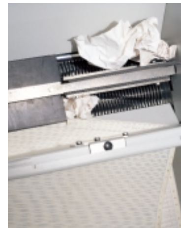
Automatic mechanical feeding system with revolving flaps
