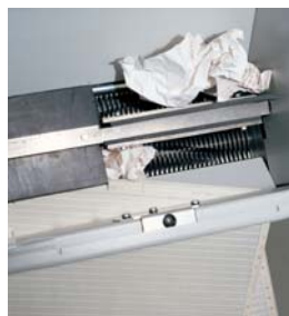
Automatic mechanical feeding system with revolving flaps
